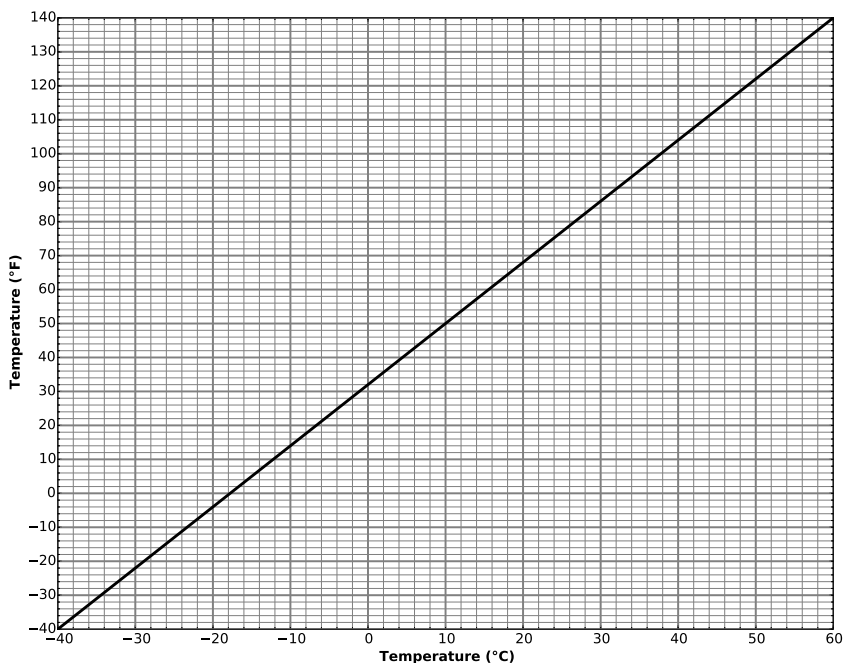
FIGURE 5-1 TEMPERATURE CONVERSION BETWEEN FAHRENHEIT AND CELSIUS
