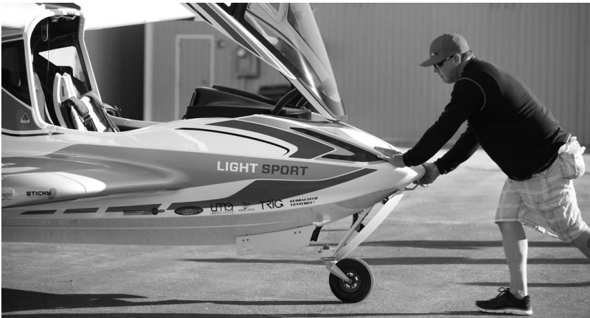
FIGURE 8-1 APPROPRIATE GROUND HANDLING TECHNIQUE
