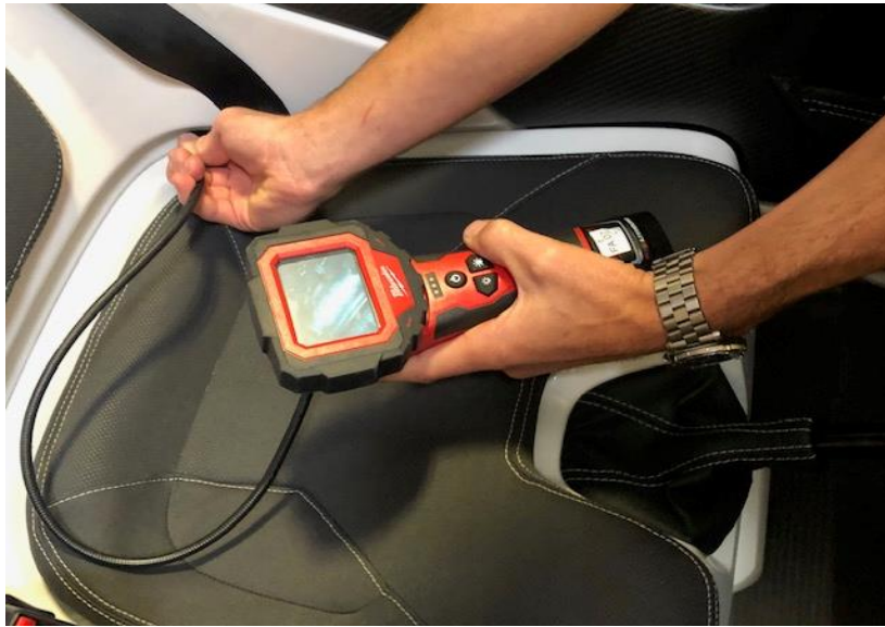
Figure 3: Borescope inspection technique though the pilot side lap belt pass through
